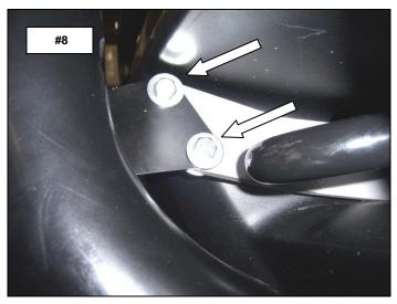
**Step-5** Align the Rhino Charger bar, bracket assembly and tighten all nuts and bolts. Remember to check and re-tighten the hardware periodically.
